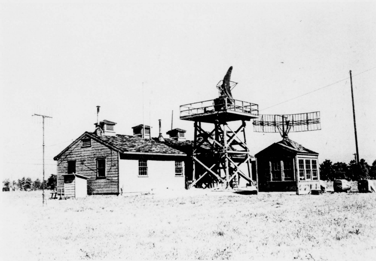
E/W - Typical early warning radar station showing AN/TPS-10A height finder on left and AN/TPS-1B search radar on right.
