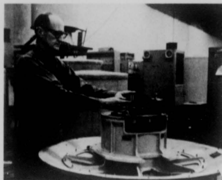
John W. Davis is shown aligning the bull gear on the TACAN drive assembly.
