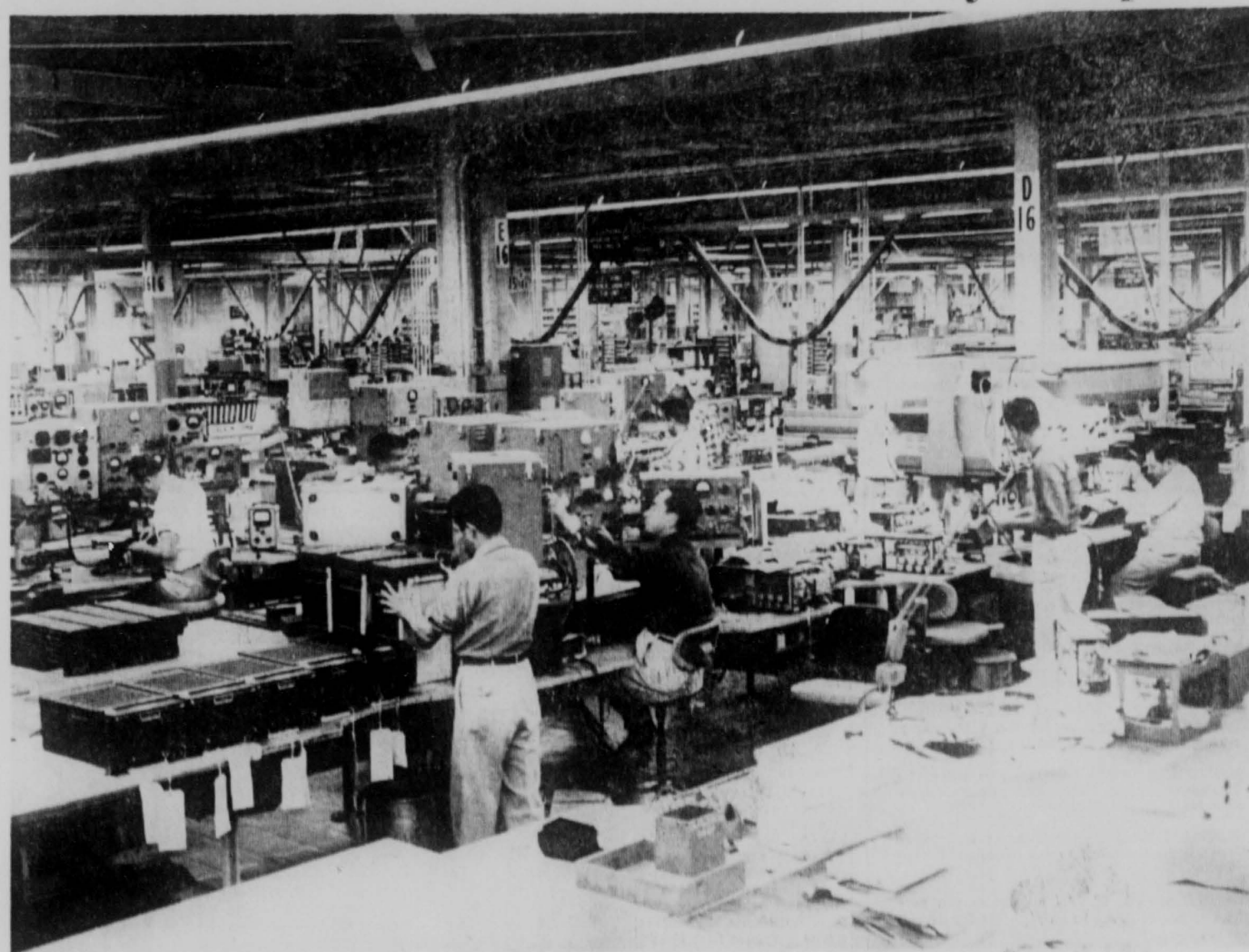
Electronics personnel maintain, modify and overhaul complicated and intricate airborne radio and radar systems.
