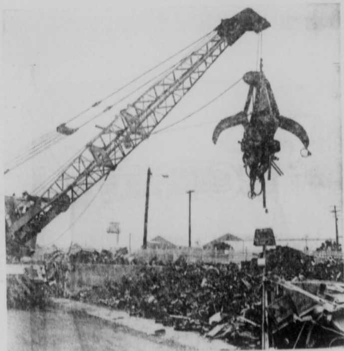
A GIANT CRANE with grapple magnet is used to pick up scrap metal at Kelly Air Force Base. The new equipment saves time and space.
