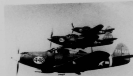
P-39Qs stacked up in echelon. The last model produced prior to the P-63, the "Q" is readily identified by the machine guns mounted in pods under the wings. The P-39Q was the first Bell fighter to employ the interconnected throttle-prop pitch concept. With this system, propeller rpm changed with throttle adjustment. Some pilots liked it, some didn't, but most never got used to it. Smithsonian Institution
