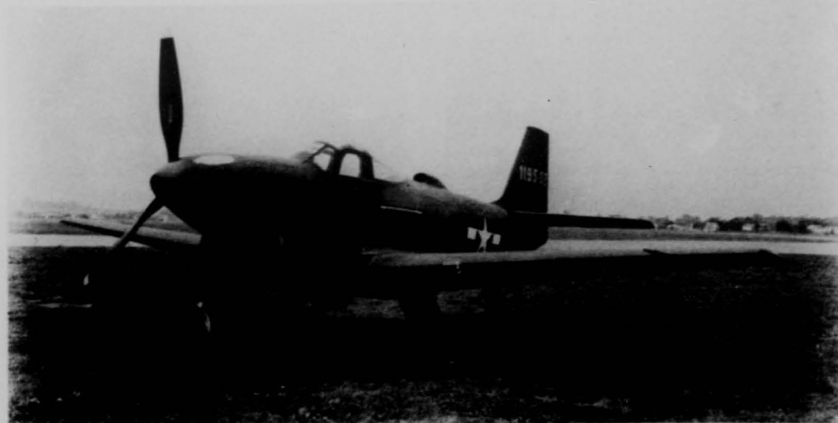
One of the many Airacobra modifications, the P-39E was test bed for the forthcoming P-63. Heaviest of the P-39 models, it grossed out at a whopping 8,918 lbs. It was powered by the Allison V-1710-47 rated at 1350 hp, the highest powered Bell
