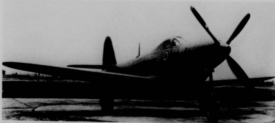
The original Pinball. Lt. Col. Donald B. Russell selected the P-63 as the frangible gunnery target aircraft mainly because it was available for training without degrading our combat efforts, and because it bore a close head-on resemblance to
