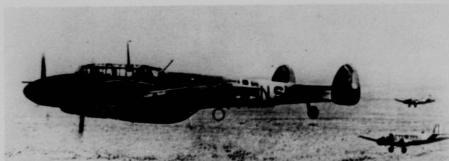
The twin-engine Messerschmitt Bf 110 proved a formidable adversary to our bomber formations over Germany and Italy. The "C" model had a 37 mm Flak 18 gun, two 20 mm cannons and three 7.9 mm machine guns firing forward. The 110 lost
