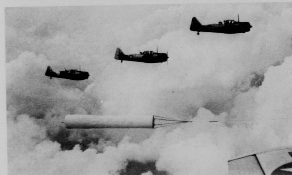
Three AT-6s carrying students on a training mission at Laredo Army Air Field. Sleeve targets (banners were also used) were towed by a variety of aircraft, usually B-17s or B-34s. US Air Force
