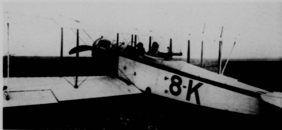
Gun cameras were used for flexible gunnery training as long ago as the early twenties. In this crude adaptation, what appears to be simple box camera may be seen just ahead of
