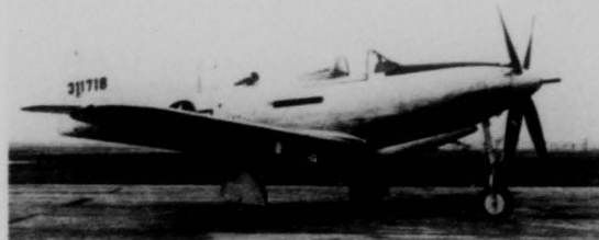
The P-63D, only Bell fighter fitted with the popular bubble canopy. Only one model "D" was built. Note machine gun pods under wings and adjacent external tank hangers. This was typical P-63 configuration. US Air Force
