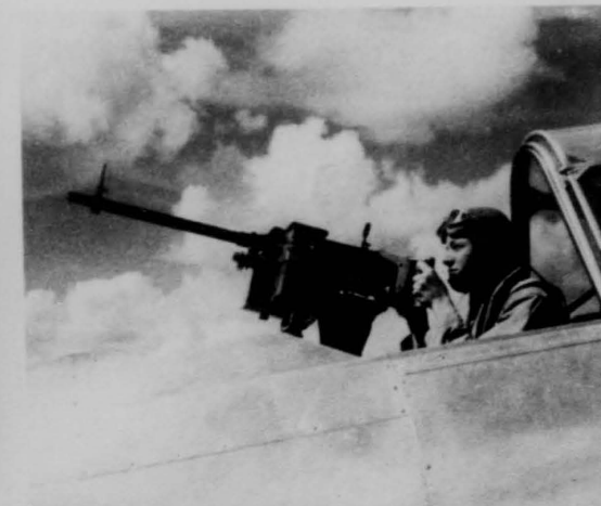
Student gunner behind a .30 caliber machine gun in the rear seat of an AT-6. Ammunition fed from metal container on left side with another on the opposite side to catch the links. Note the canvas bag on bottom designed to pick up spent cartridge casings. US Air Force
