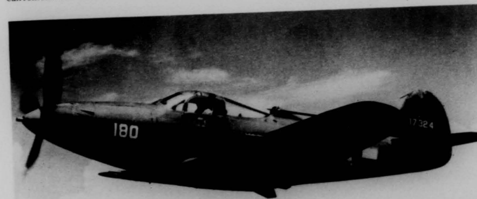
The P-39F was basically a P-39D with minor modifications. An Aeroproducts constant speed propeller was substituted for the Curtiss-Electric and this improved reliability. Only
