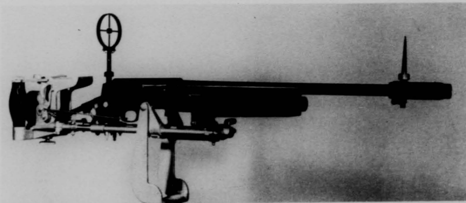
The Browning 12-gauge automatic shotgun as it was adapted for skeet shooting from a pedestal. With this adaptation, stock has been replaced with machine gun-type handles. Note
