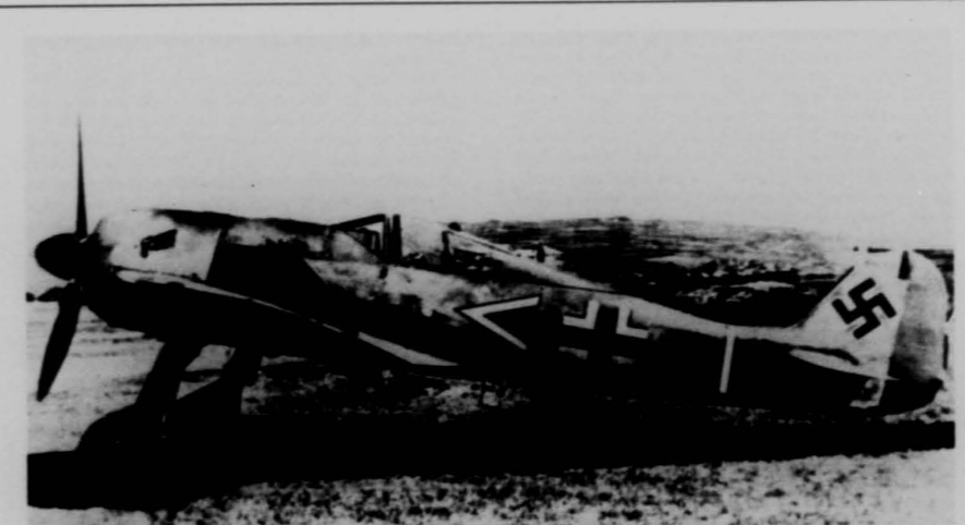
The Focke-Wulf FW 190 was a fine fighter with a BMW air-cooled radial engine that in later versions exceeded 2000 hp. The FW 190 was heavily armed and, with its wide landing gear was much easier to land than the Bf
