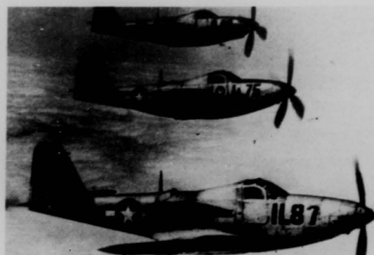
Three RP-63As stepped up in echelon. These pinballs display two types of carburetor air intakes. The middle aircraft has a flush intake, the other two sport the clamshell type. Ernest R. McDowell
