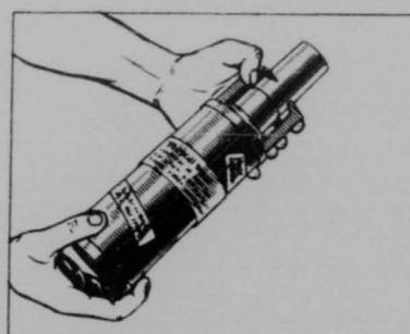
(2) REMOVE FUZE FROM SEALED CONTAINER (IMPORTANT—KEEP THE CONTAINER IN EVENT FUZE HAS TO BE REPACKED)
