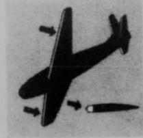
**LEADING EDGE** — The part of an airfoil which strikes the air first.
