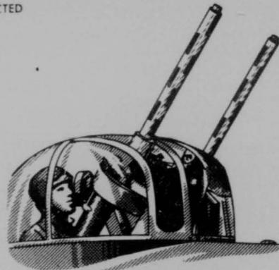
Figure 1-2. Topside, Twin Fifty-Caliber Colt-Browning Guns in a Power Turret on a B-25.
