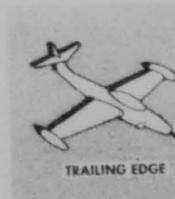
**TRAILING EDGE** — The rear or following edge of an airfoil such as a wing or propeller-blade.
