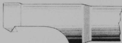
Figure 2-75. Firing Pin Extension Showing Worn Notch, Dotted Line Indicates Satisfactory Notch.
