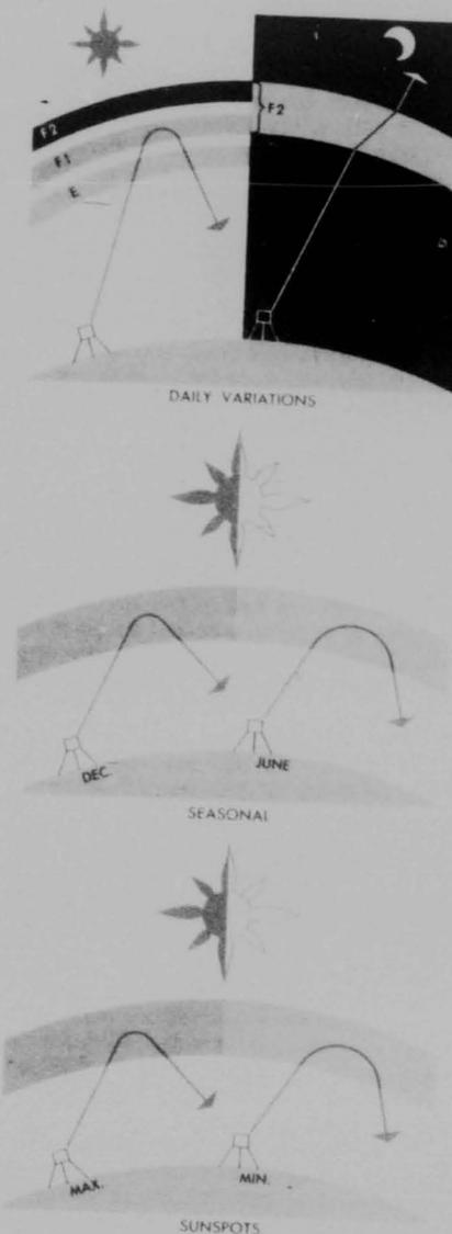
Figure 3-69 Predictable Ionospheric Variations
