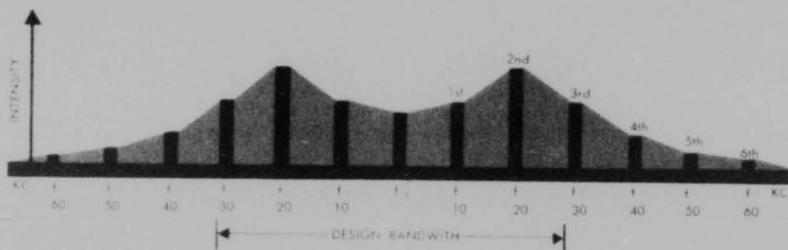
Figure 3-18 Spectrum Distribution for Modulation Indices
