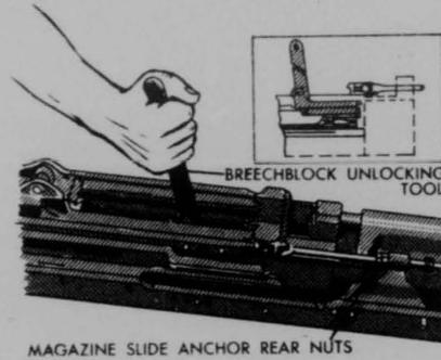
Figure 1-26. Positioning Breechblock Unlocking Tool in Gun.
