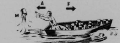
PRINCIPLE OF REACTION - THE DIFFERENCE BETWEEN JET PROPULSION AND ROCKET PROPULSION
