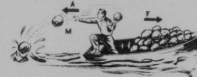
PRINCIPLE OF REACTION - SECOND PHASE - "FOR EVERY ACTION THERE IS AN EQUAL AND OPPOSITE REACTION"
