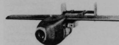
The control surfaces are actuated by radio signals transmitted by the bombardier of the launching airplane. The bombardier tracks the bomb by means of a television set in the nose of the bomb which enables him
