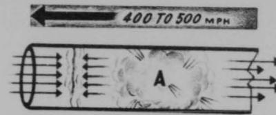
Figure 9-6. Ram-Jet Operation—Moving at 400-500 MPH. There is a Head of Air in the Front of the Pipe Which Resists Expansion (Acceleration) in That Direction.
