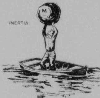
PRINCIPLE OF REACTION - FOURTH PHASE - "A BODY AT REST HAS INERTIA AND THEREFORE WILL RESIST MOTION AND PROVIDE 'PUSH' AS ILLUSTRATED IN (FIG 9-27)"
