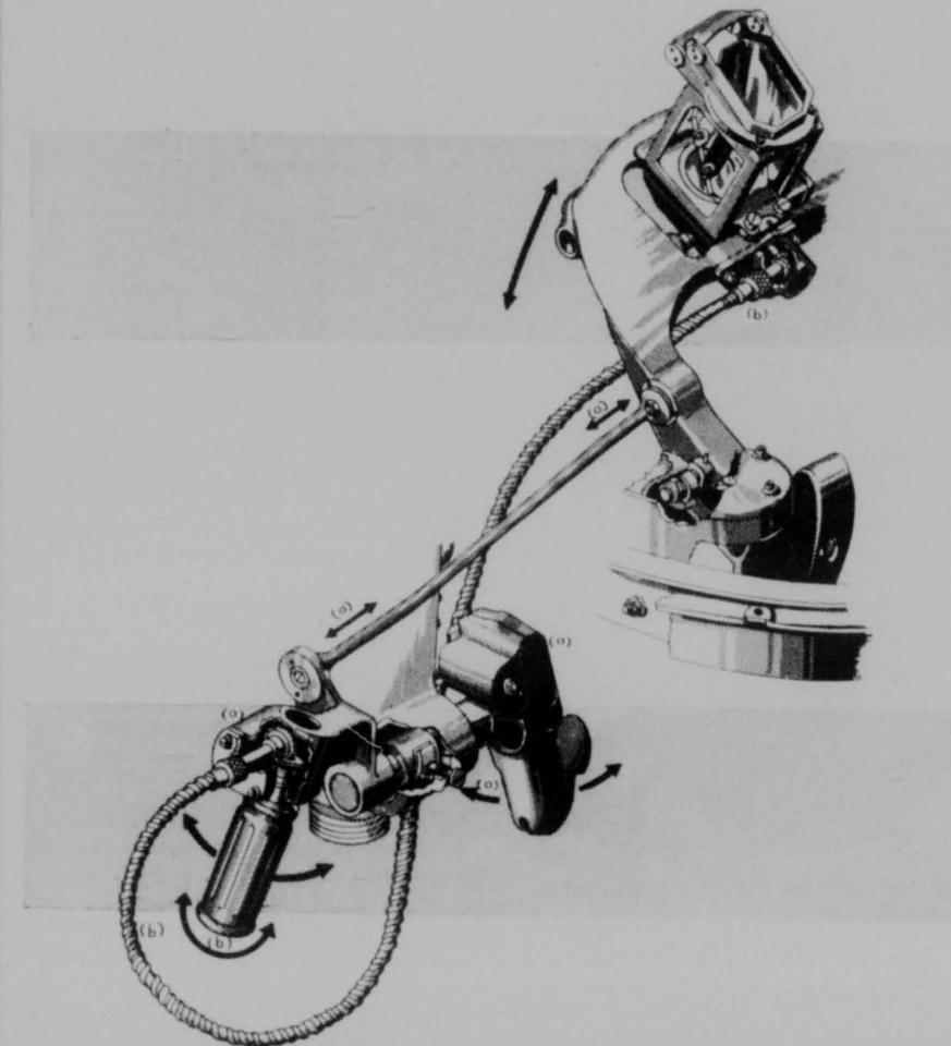
Figure 6-50. Schematic Diagram Showing How the Control Grips are Linked to the Yoke, and How the Range Grip is Connected to the Sight.
