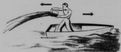
As a result the boat will move along, just as a jet aircraft moves along. It moves because he (the engine) is pushing against (accelerating) a mass of water; and not because the water he is hurling is pushing on the air or on anything else. This is the important part of the whole reaction-propulsion idea.
