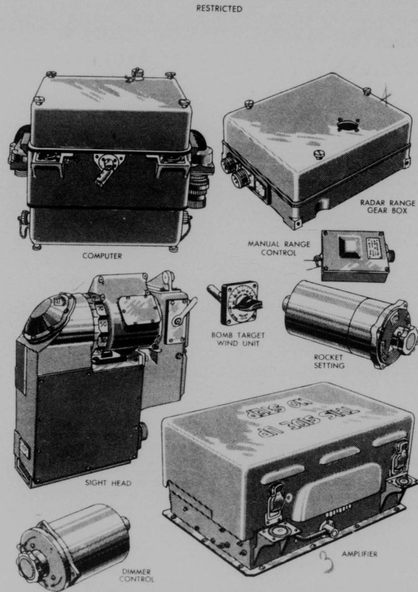
Figure 4-1. Type A-1B Sight (Gun-Bomb-Rocket) Components
