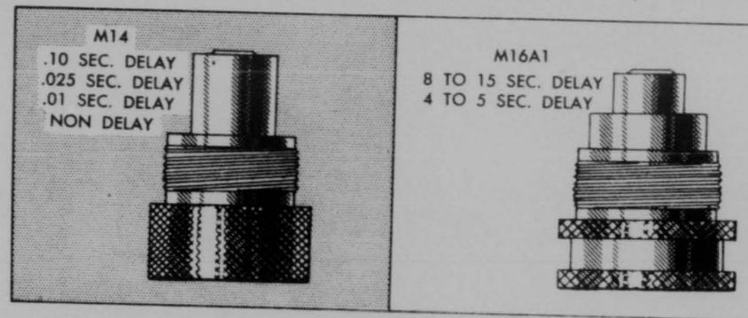
Figure 7-10. Short and Long Delay Primer Detonator.
