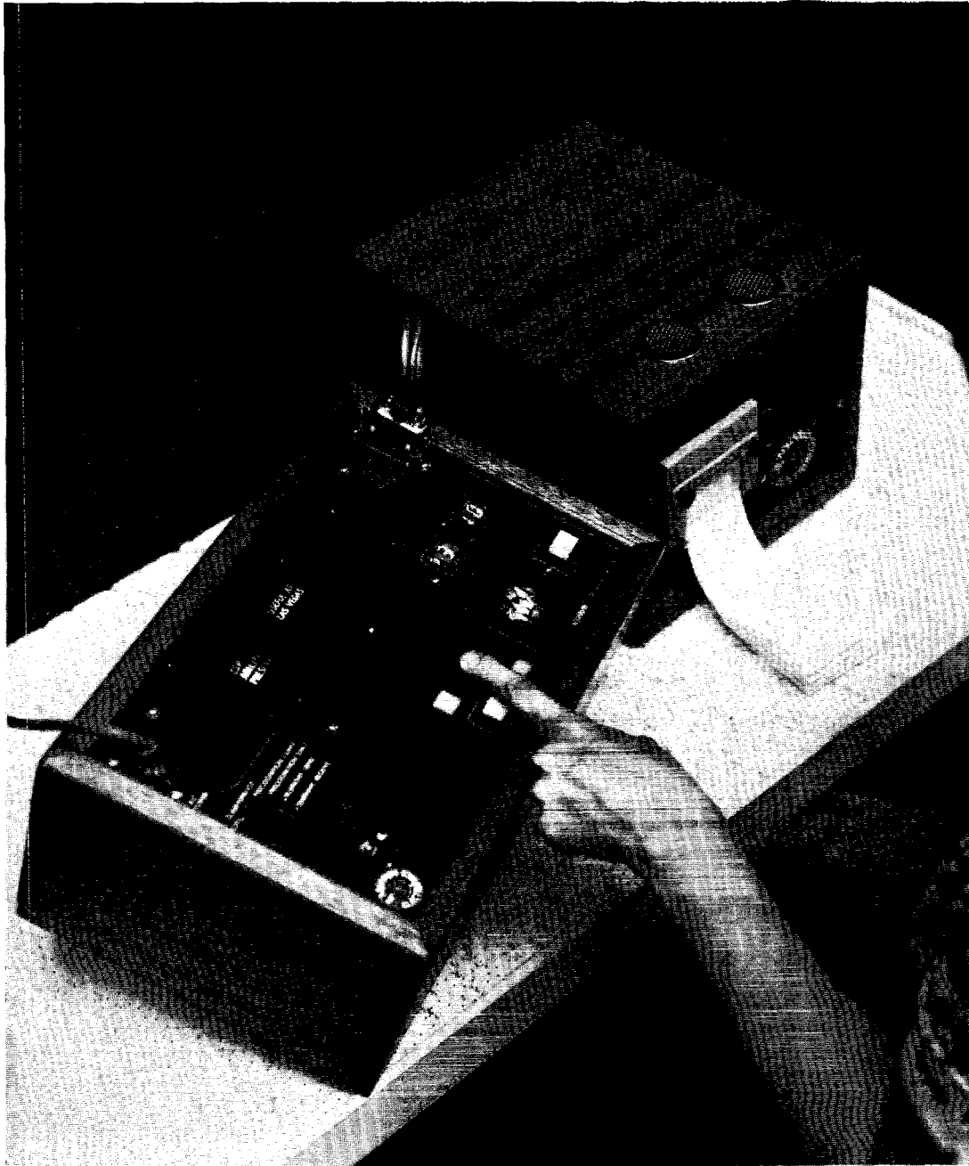
Figure 3. ESP Teaching Machine used in this experiment. An incorrect choice of target is indicated. Two of the five "encouragement lights" at the top of the machine are illuminated. The printer to the right of the machine records data on fan-fold paper tape.
