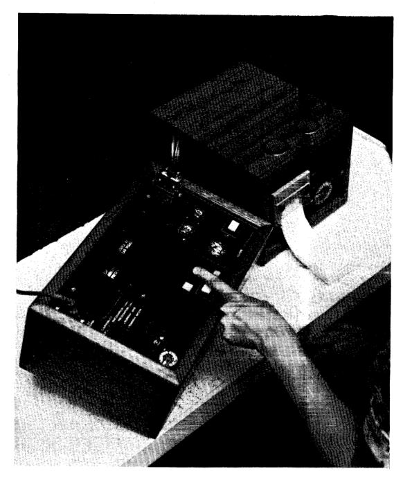
Figure 8. ESP Teaching Machine used in this experiment. An incorrect choice of target is indicated. Two of the five "encouragement lights" at the top of the machine are illuminated. The printer to the right of the machine records data on fan-fold paper tape.
