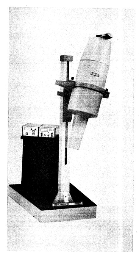
SUPERCONDUCTING DIFFERENTIAL MAGNETOMETER
