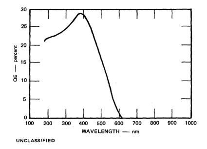
FIGURE 2 (U) SPECTRAL RESPONSE OF 9829 QB PM TUBE
