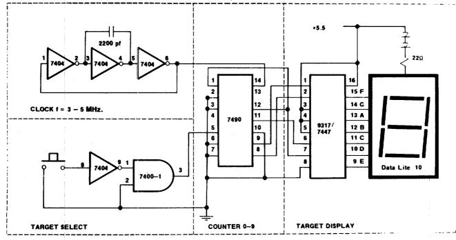
Circuit of the random number generator (RNG) used to generate targets for the TCT. Fig. 5. Integrated circuits are Signetics types 7404, 7400, 7447, and 7490. Seven segment display is a Litronix Data Lite 10.
