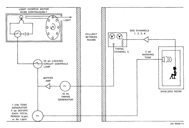
FIGURE 2 SCHEMATIC OF THE REMOTE SENSING EEG EXPERIMENT
