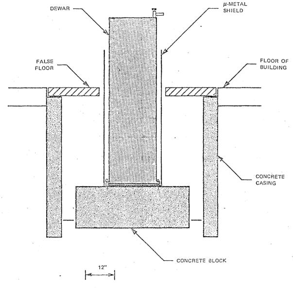
FIGURE 1 MAGNETOMETER HOUSING CONSTRUCTION
