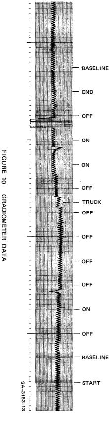
discussed below. An artifact due to the passage of a truck in the parking lot adjacent to the laboratory (under continuous surveillance by the experimenter) is noted in period 6. Each of the signals on scale  $\frac{\text{corresponds to}}{\text{corresponds to}} \text{ an input } \sim 1.6 \times 10^{-9} \text{ Gauss/cm}^2 \text{ (second derivative } \delta^2 \text{B}_z/\delta^2_z),$  which is equivalent to  $\sim 3.5 \times 10^{-7}$  Gauss referred to one pickup coil.
