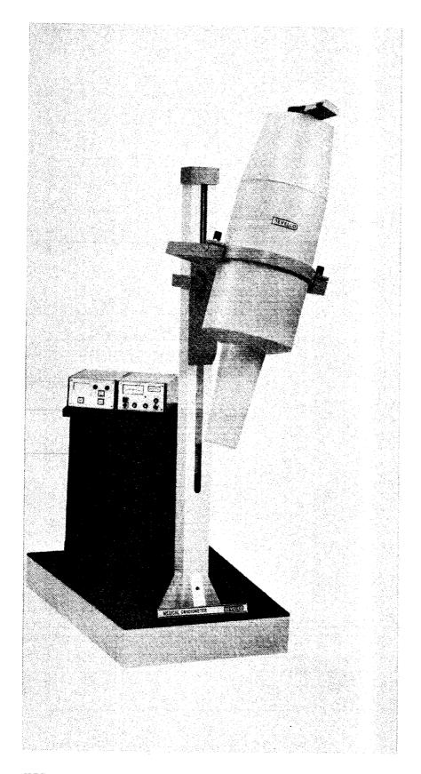
FIGURE 9 SUPERCONDUCTING DIFFERENTIAL MAGNETOMETER
