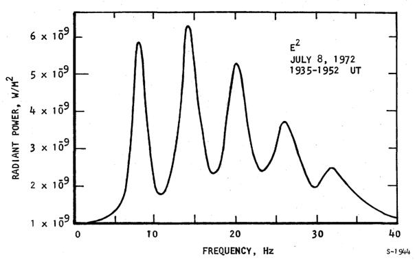
Figure 7-4. High-Resolution Measurement of Schumann-Wave Radiation Near Kingston, R.I. (After Reference 7-2, p. 40).
