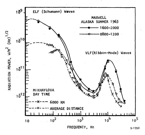
Figure 7-5. Measured Atmospheric "Noise" in the ELF and VLF Regions (After Reference 7-2, p. 42).
