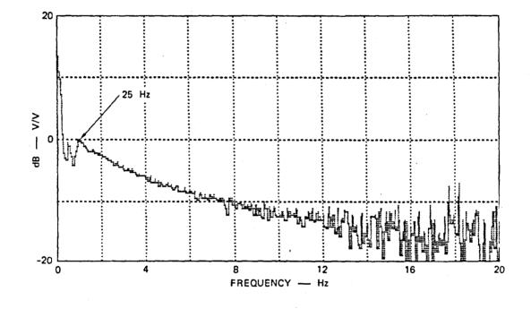
FIGURE B-9 TRANSFER FUNCTION FOR THERMAL PULSE
