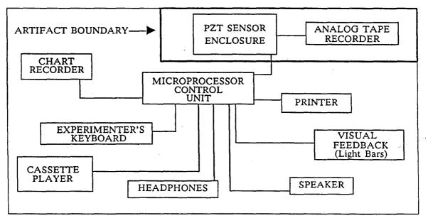
FIGURE 2 DIAGRAM OF RA APPARATUS
