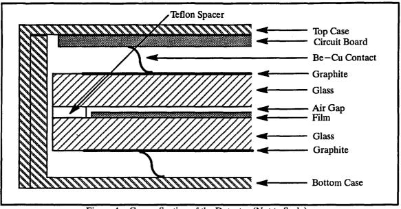
Figure 4. Cross-Section of the Detector (Not to Scale).
