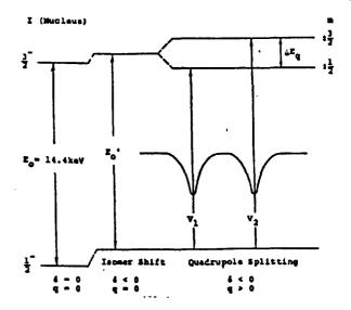
Figure 5. Electric Quadrupole Splitting
