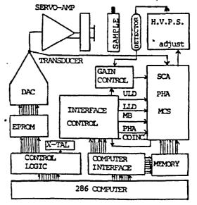
Figure 7. Block diagram of spectrometer
