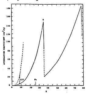
Figure 8. Attenuation coefficient for 14.4keV gamma radiation as a function of element.
