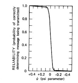
Fig. 19. Reliability curve for sequential sampling procedure ( $p_0 = 0.4$ ,  $p_1 = 0.6$ ,  $\alpha = 0.01$ ,  $\beta = 0.01$ ).
