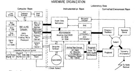
Fig. 1. General layout of the research facility. (Heavy arrows denote multichannel data paths; dashed vertical lines delimit physically separate regions of the facility.)
