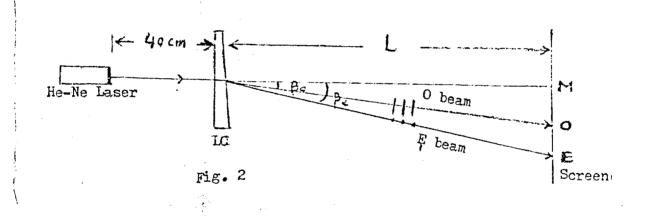
In fig.2,  $\beta_o$ ,  $\beta_e$  are the angles of deflection of 0 beam and E beam respectively. L is the distance between the laser and the LC. MO and ME are the distances of deflection of two beams from the horizontal line on the screen.
