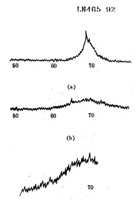
ILLUSTRATION THREE: X-RAY DIFFRACTION SPECTRAL LINES OF THREE PIECES OF MONOCRYSTALS PROCESSED FOR EXTRACTION
