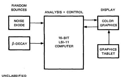
FIGURE 1 (U) BLOCK DIAGRAM OF COMPUTER-BASED RNG SYSTEM
