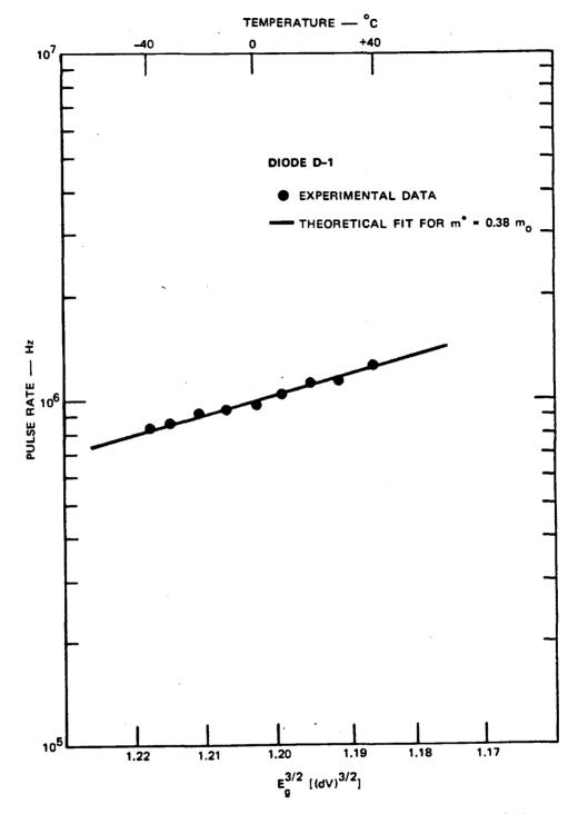
Figure 3. Log of the pulse rate as measured by frequency analysis plotted as a function of band gap.
