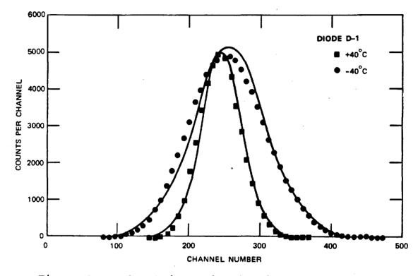
Figure 2. Pulse height distribution of filtered diode noise from -40 to +40°C
