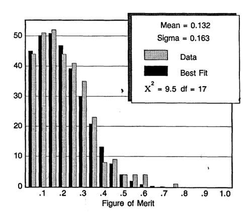
Figure 1 BEST-FIT GAUSSIAN TO CONTROL FMs
