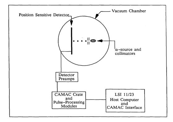
FIGURE 2 SINGLE *α*-PARTICLE RA APPARATUS
