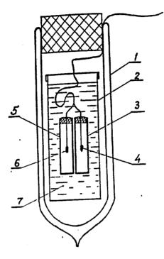
Fig. 2.1. Design of the screened microcalorimeter. 1--Dewar Flask, 2--glass, 3 and 5--shells, 4--thermistor, 6--temperature stable resistor, 7--melting ice.
