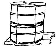
\* Barrels stoched two high in groups of 3; each group is secured together. - These pallets of 6 bands are then stacked for high themselves - Bands are parit/ green w/ no exterior markings. - Centain a liquid chemical highly toxic & dangerons. - Chemical is poisonous to humans, but its purpose is not specifically to poison or gas humans.
