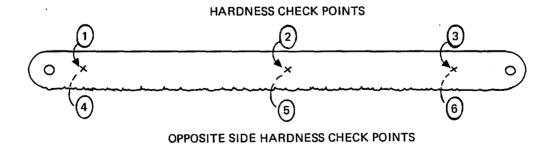
Figure 1. Hardness Test Point Areas
