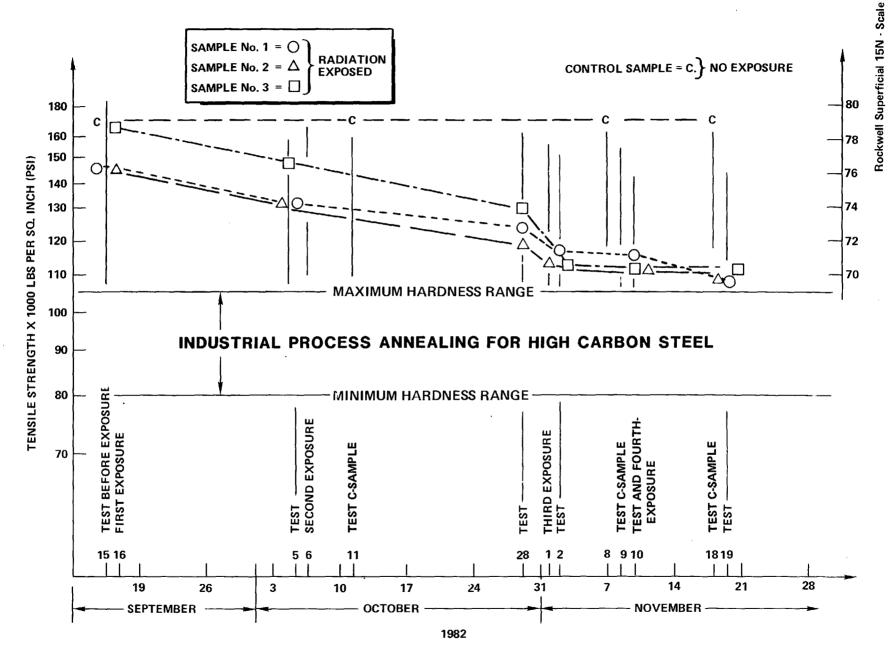
FIGURE 2. STRENGTH REDUCTION BY REMOTE ANNEALING RADIATION (RAR) FOR HIGH CARBON STEEL HACKSAW BLADES
