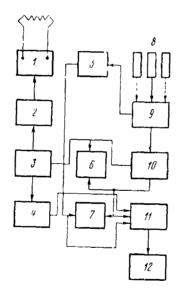
Fig. 1. A block-diagram of the set up for investigating the drift of the small scale irregularities in the ionosphere.
