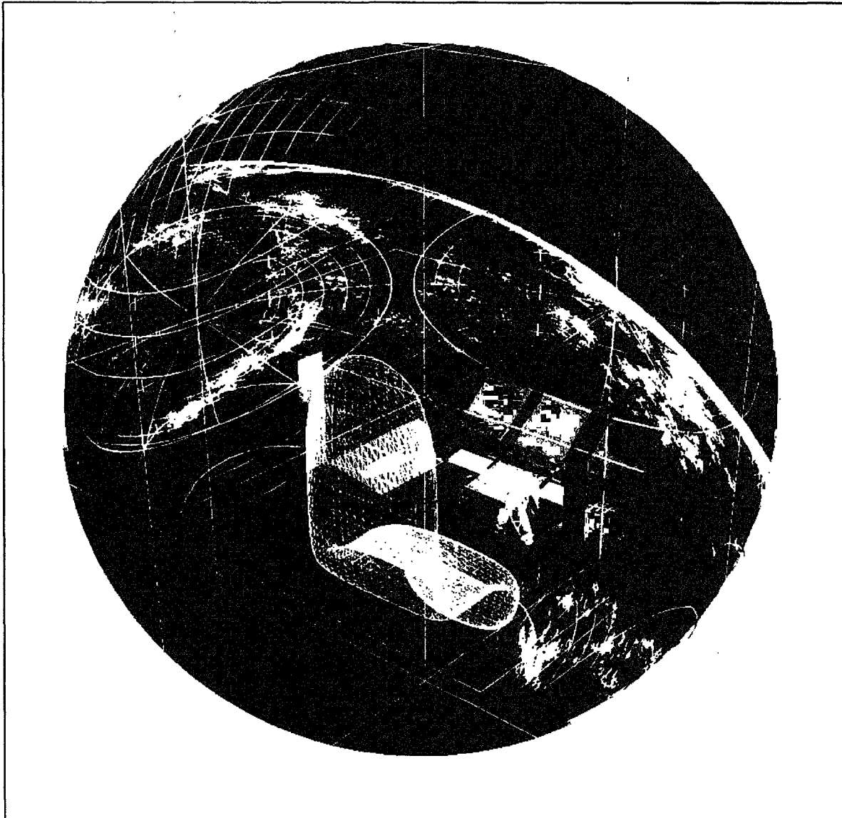
Figure 13. Provisional Breakthrough-Era Cockpit. The spherical zone around the cockpit center represents the virtual surround display onto which images of the environment outside the vehicle are displayed. Keeping with lessons of prior human interfaces, a minimal set of physical displays are also provided, with the most important ones located deliberately in the "tunnel vision" zone in front of the pilot. [Graphic: A. Szames with background image through M. Cherfi]
