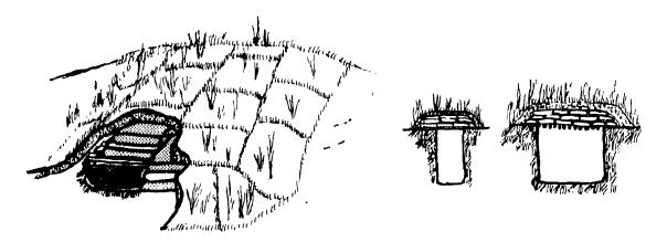
FIGURE 9. PROTECTING SANDBAGS WITH SOD AND EARTH COVER.
