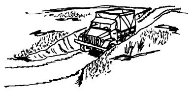
FIGURE 22. PROTECTION OF VEHICLES IN SLOT TRENCHES.
