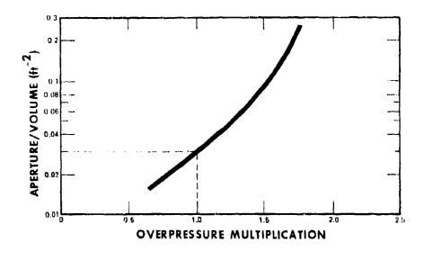
FIGURE 10. OVERPHESSURE MULTIPLICATION PLOTTED AS A FUNCTION OF OPENING/VOLUME RATIO.
