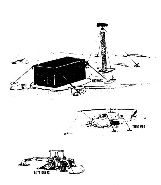
FIGURE 17a. ANCHORS, TIEDOWNS, AND OUTRIGGERS.
