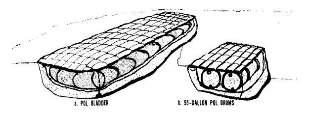
FIGURE 28, PROTECTING POL BULK STORAGE CONTAINERS.
