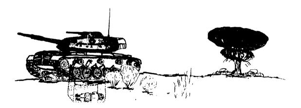
FIGURE 7. USING TRACKED VEHICLES AS EXPEDIENT OVERHEAD COVER.
