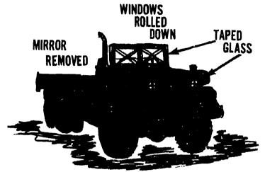
FIGURE 20. PROTECTING VEHICLE GLASS.
