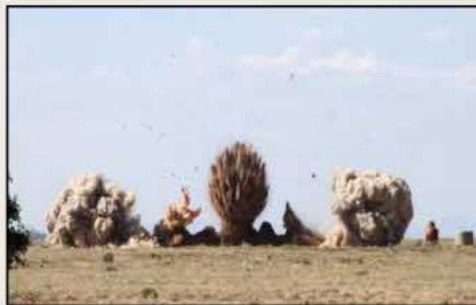
10-ton ANFO on Alluvium Lithology (top) and Tunnel Shot (bottom) Yield Estimation Sensor Tests
