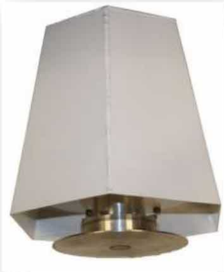
Figure 1 – OPS System Showing Transducer at the Center of the Lower Disk (aka the Turbulence Mitigation Plate).
