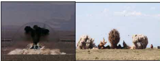
10-ton ANFO on Alluvium Lithology (left) and Tunnel Shot (right) Yield Estimation Sensor Tests
