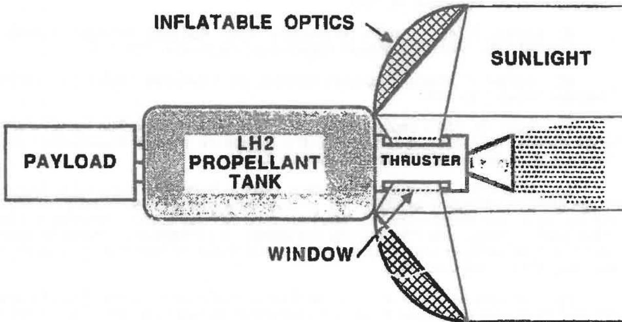
Figure 8-1 Solar Thermal Propulsion Concept
