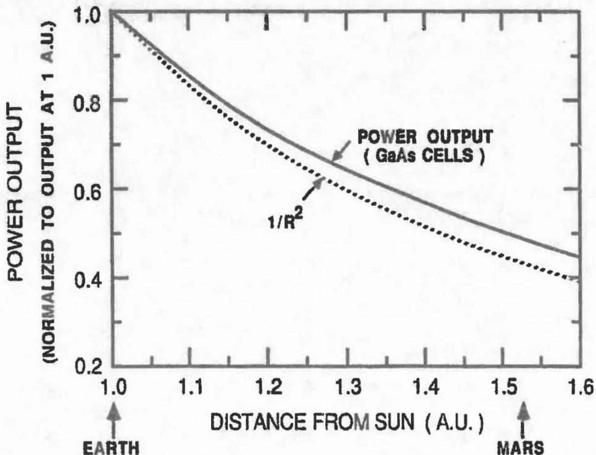
Figure 3-2. Solar Photovoltaic Array Power Output vs. Distance from the Sun
