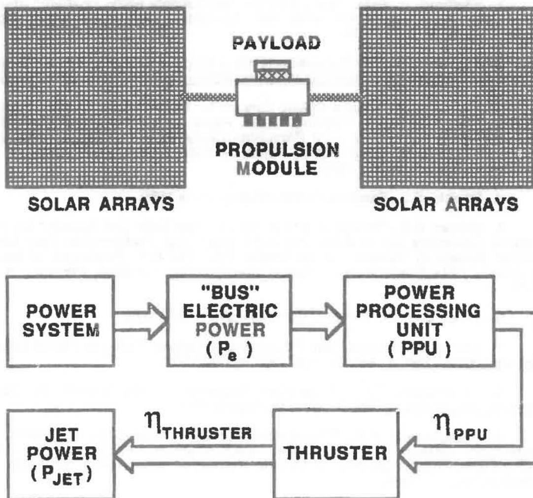
Figure 3-1. Solar Electric Propulsion (SEP) Concept
