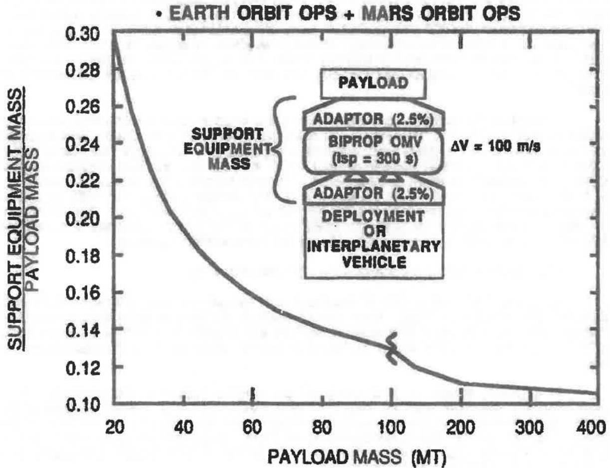
Figure 1-3. Effective Payload Weight Due to Adding an Orbital Maneuvering Vehicle (OMV) for Earth and Mars Orbital Operations
