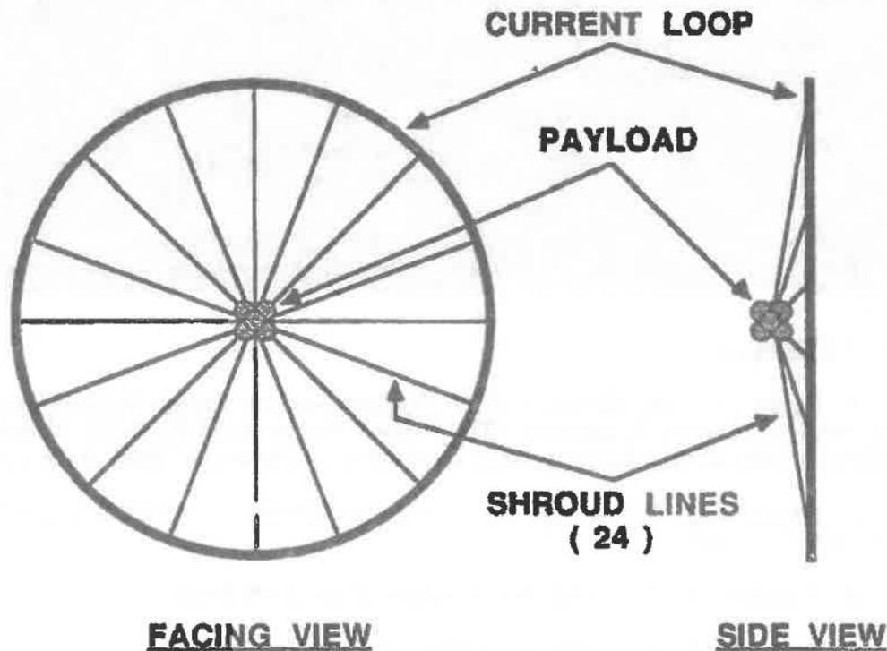
Figure 5-1. Magsail Deployed With Payload, Normal Configuration
