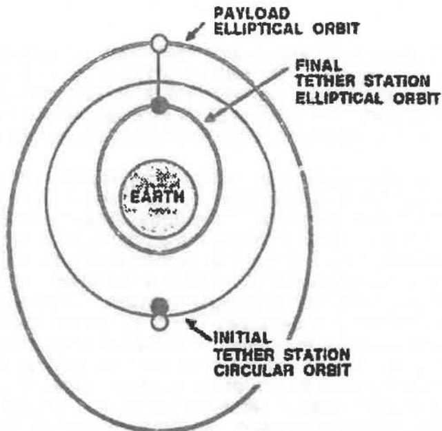
Figure 9-1. Tether System Orbits at Earth
