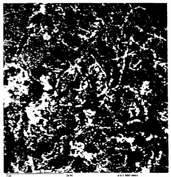
SEM image showing gold acting as a solder to form strong attachments between nanotubes in order to produce an ultra-strong, lightweight material
