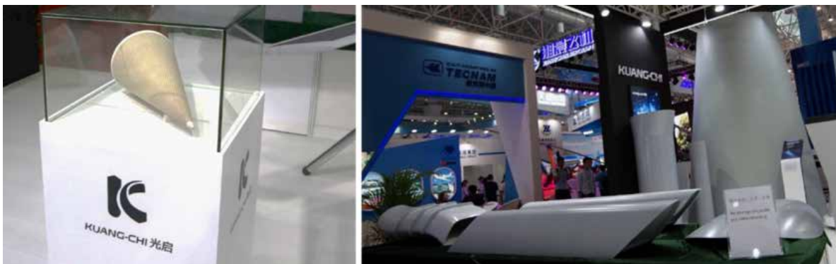
Frequency Band Pass Radar Nose Cone and Other Aircraft Structures Made of Meta-Materials Displayed at AirShow China 2018 177
